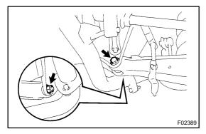
(f) Remove the bolt, nut, washer and No.2 lower suspension arm.
