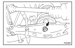
(c) Remove the bolt, nut and disconnect the shock absorber from the No.2 lower suspension arm.
