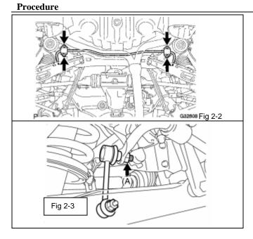
(b) Install the rear stabilizer bar with the 4 bolts. (Fig 2-2)
