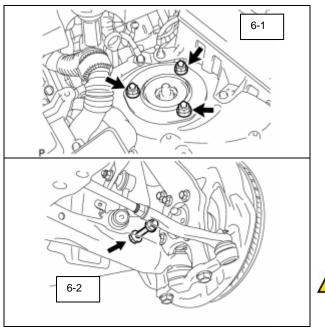
(b) Insert the bolt from the rear of the vehicle, and install the front shock absorber lower side on the front lower suspension arm. (Fig 6-2)
