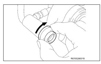
Rotate the dust boot to spread the Toyota White Grease or lithium soap base glycol grease evenly.
