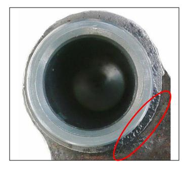
• Specks appear after rust has been removed. This is normal; no further action necessary.
