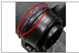
e) Verify that Toyota White Grease or lithium soap base glycol grease extrudes from between the brake caliper and the dust boot.
