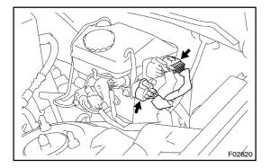
(a) Disconnect the 2 connectors from the hydraulic brake booster. (b) Connect the actuator checker (SST) to the hydraulic brake booster side wire harness via the sub-wire harness (SST), as shown in the chart below.
