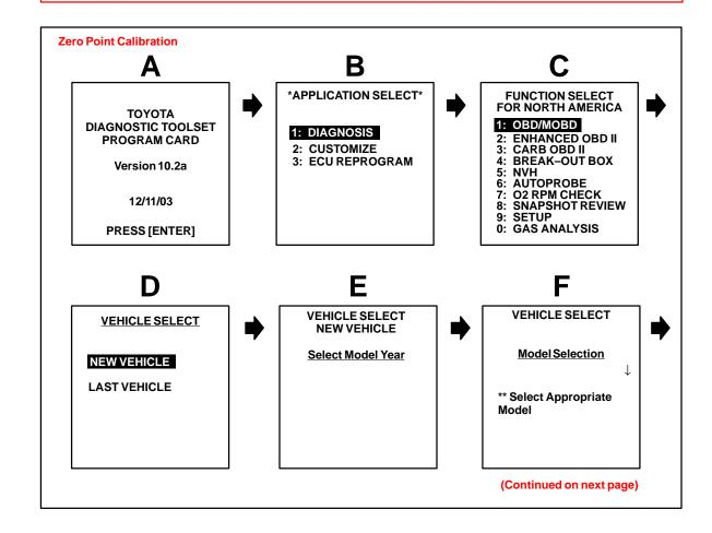
Calibration Procedure With Diagnostic Tester (Continued)
