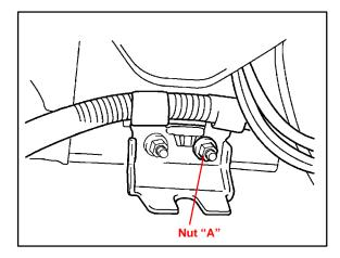
F. Install the terminal of the luggage compartment ground wire with the new nut, as shown in the illustration.
