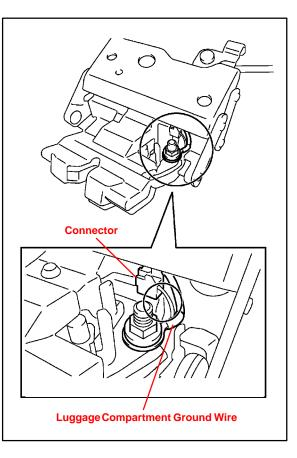
C. Secure the luggage compartment ground wire with a cable tie.
