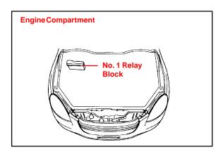
2. During PDS, install the D/C CUT fuse in the No. 1 Relay Block as shown.
