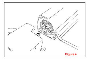
C. Install the bracket to the tonneau cover retractor holder and tighten the 3 screws.
