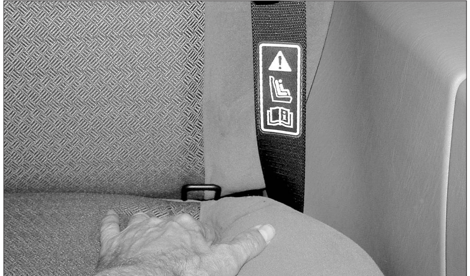
Figure 5—By pushing down on the lower half of this rear seat, the lower anchor for the child safety seat can be seen.
