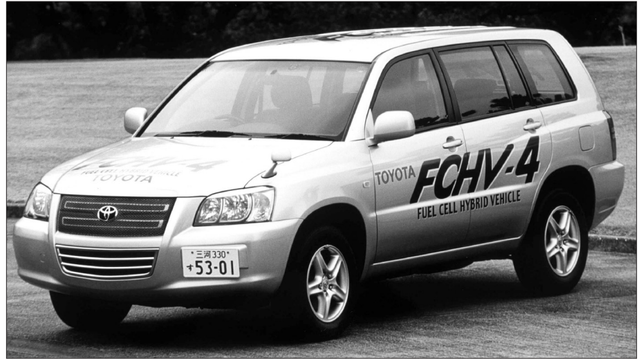
Figure 4–Toyota's FVHV-4, the latest in a series of Fuel Cell Hybrid Vehicles, stores hydrogen in high-pressure tanks. (Courtesy of Toyota Motor Corporation)
