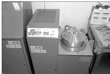
Figure 3—The solvent recycling equipment must be located in an area that meets all local code requirements.
