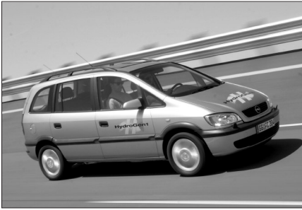
Figure 3–The only materials coming from the exhaust pipe on the GM Hydrogen 1 fuel cell concept vehicle is pure water vapor. (Courtesy of General Motors Corp.)
