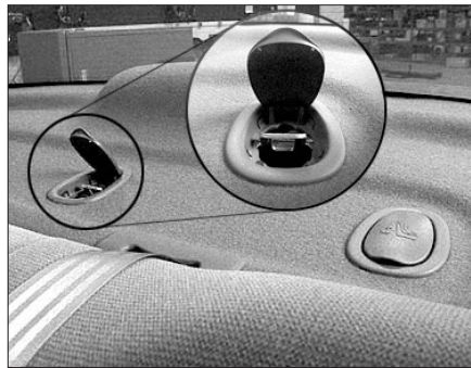
Figure 3—The top tether anchor allows a child safety seat strap to be attached.
