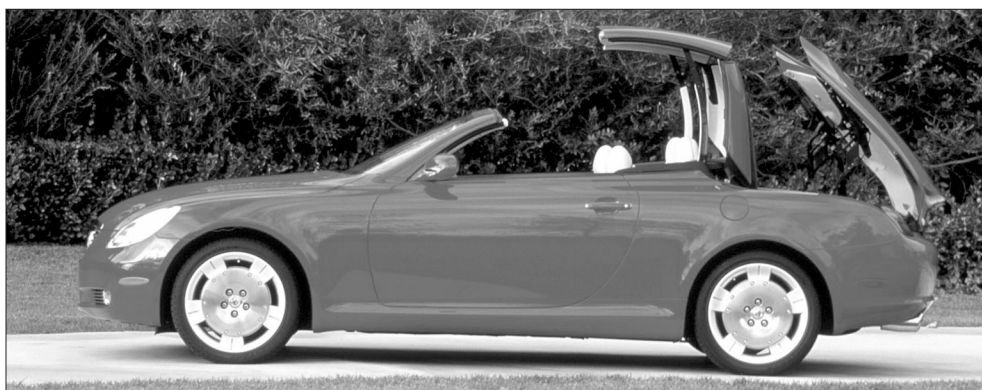
The retractable roof on the Lexus SC430 opens and stores in the luggage compartment with the touch of a button.
