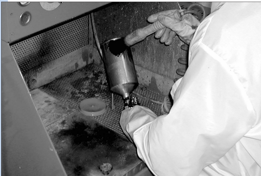
Figure 1—The practice of cleaning spray guns uses more solvents than any other process in a collision repair facility.
