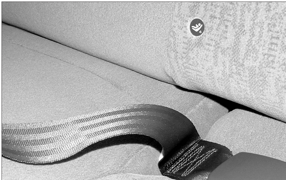
Figure 4—The icon in the circle on the lower rear seat indicates that there are lower anchors for a child safety seat located below the crack of the seat.
