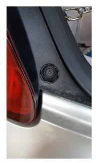
Remove the one #2 Philips screw. Then pull out the tail light assembly. Read on first....
