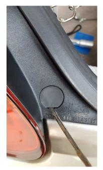
Open the trunk to expose the screw cover, which is technically on the outside of the trunk, but cannot be accessed without the trunk open. Remove the cap with a small flat blade screwdriver.
