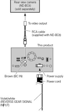
For more details about the wiring, refer to Connecting the power cord on page 67.
