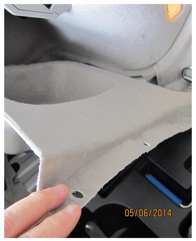
This is a view of the back panel. I put a spare tire kit in my SC430 so it may look slightly different if you are using run flats. Remove all the clips, tie downs, and rubber bumpers.
