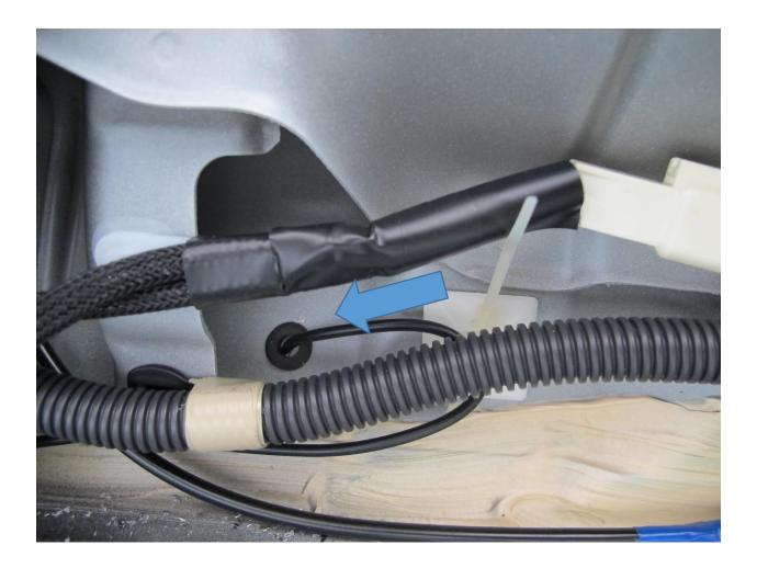
I slipped some 3/8 inch cable tubing from home depot to protect the camera wire. It matched the OEM tubing and will protect the wire.
