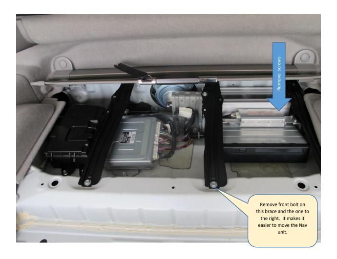
Now you can see the top module unbolted and I was able to sit it on top of the unit behind it when accessing the Navigation unit connectors.
