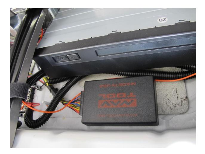
Here is my tap to the backup light on the passenger's side. You can just pry open the cable conduit and pull the wire out. Once taped I just pushed it back in and used some electrical tape to make sure it was secure. I then tested that I had 12v here when the car was put into reverse.
