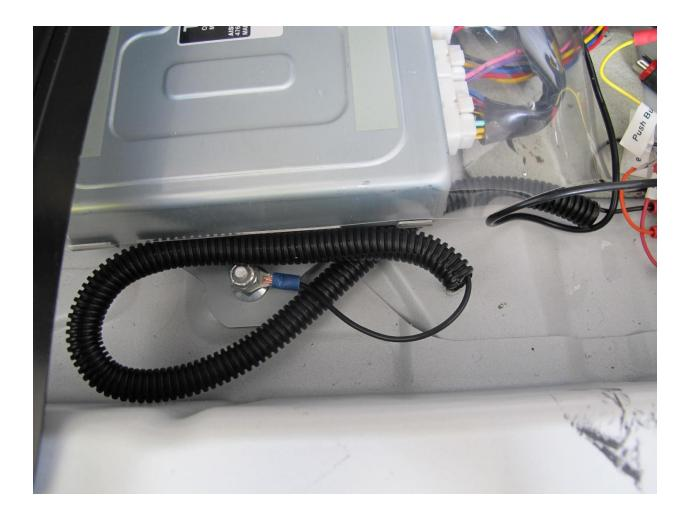
I used a terminal strip I purchase at radio shack to distribute 12v and ground. Originally I put the reverse connection there also but this got me into issue #2 which still puzzles me. I'll cover this later. Anyway this was easier than multiple splices and will make it easier to trouble shoot in the future.
