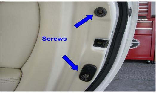
Once the clips are removed, remove the bezel from the door handle, remove the screws, and take out the door switch panel. Insert a small screw driver (covered with masking tape) and push on the clip and lift slowly. Disconnect the two connectors.
