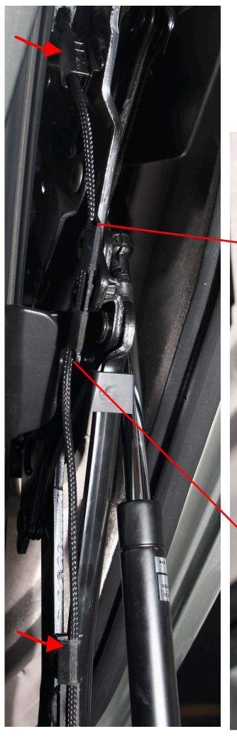
The sheath is secured to the hinge with velco straps in a few place.
