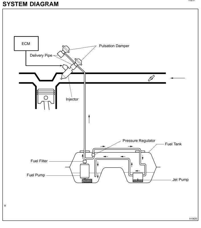
**Author:** Date: 2722 The fuel system is controlled by the ECM based on signals from various sensors.
