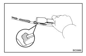
(4) Using a scraper, remove any excess or protruding adhesive.
