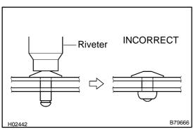
Do not have any space between the moulding outside and body panel. Firmly hold together the 2 items while installing the rivet.
