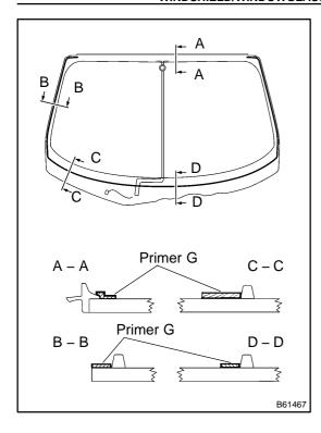
(c) Using a brush or sponge, apply Primer G to the contact surface of the glass.
