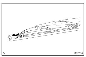
(b) Install the wiper rubber LH in the way that the head part (Longer side) of the wiper rubber faces the arm axle side.NOTICE:
