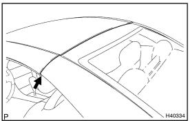
(g) Push up the roof panel and the back window near the parting line and check that they are locked.
