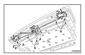
(h) Using a torx socket, fully tighten the 3 screws (b). Torque: 9.0 N·m (92 kgf·cm, 80 in.·lbf)
