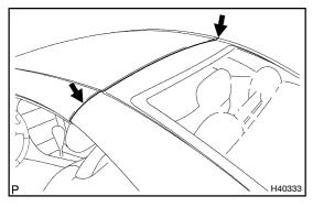
(e) Strongly push down the roof panel and back window near the parting line.
