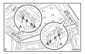
(c) Using a torx socket, remove the 8 screws.
