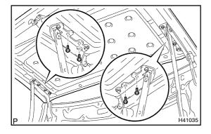
(b) Using a torx socket, tighten the 4 bolts.
