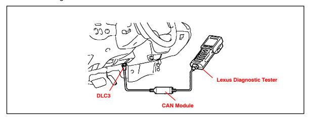
2. Follow the flow below for the calibration procedure. If the vehicle is equipped with automatic transmission (A/T), ensure that the shift lever is in the "P" range and the parking brake is applied. If the vehicle is equipped with manual transmission (M/T), ensure that the parking brake is applied.
