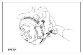
(c) Insert two sliding pins into the torque plate.
