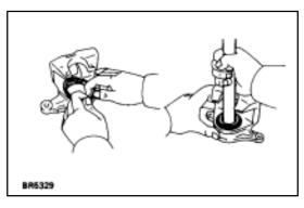
3. INSTALL PISTON SEAL AND PISTON IN CYLINDER
