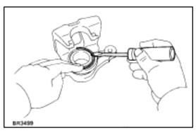
4. INSTALL CYLINDER BOOT AND CYLINDER BOOT SET RING
