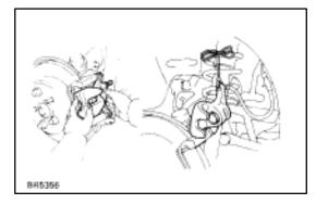
(c) Lift up the brake cylinder and suspend the cylinder with string.
