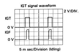
During cranking or idling, check waveforms between terminal IGT and E 1 of engine control module.
