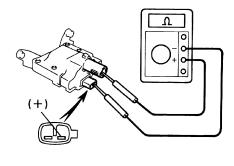
P Disconnect ignition coil connector.
