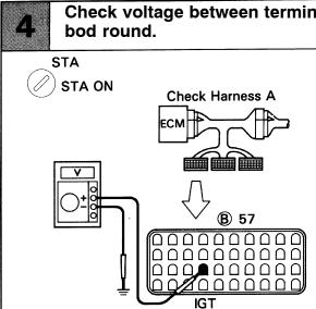
Check voltage between terminal IGT of engine control module connector and bod round.
