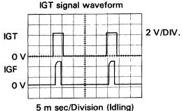
During cranking or idling, check waveforms between terminal IGT and E i of engine control module.
