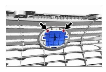
(b) Disengage the claw and guide as shown in the illustration to remove the radiator grille (or front panel) emblem.
