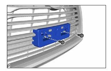
(b) Disengage the 2 claws and remove the front bumper extension moulding bracket as shown in the illustration.
