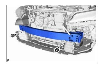
(c) Remove the 6 bolts and front bumper reinforcement sub-assembly.
