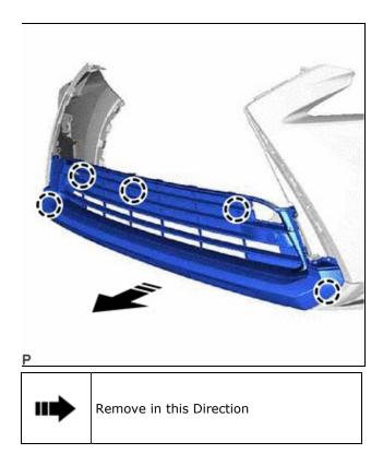
(b) Disengage the 8 claws as shown in the illustration to remove the lower radiator grille moulding.
