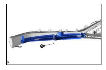
(b) Disengage the 2 claws as shown in the illustration to remove the front bumper side support LH.
