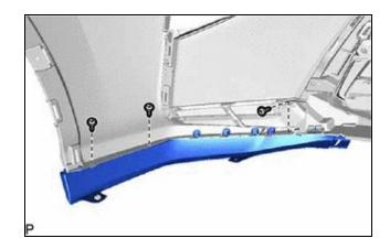
(b) Disengage the 5 claws as shown in the illustration to remove the front bumper guard cover LH.
