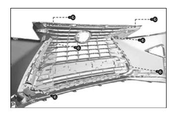
(b) Disengage the 13 claws and 4 guides as shown in the illustration to remove the radiator grille moulding.
