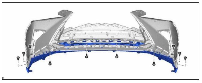
(b) Disengage the 18 claws as shown in the illustration to remove the front bumper extension.
