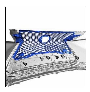
(b) Disengage the 8 claws as shown in the illustration to remove the radiator grille.
