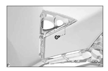
(b) Disengage the 5 claws as shown in the illustration to remove the fog light cover LH with radiator grille garnish.
