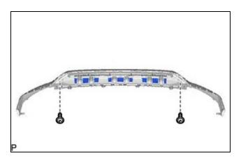
(b) Disengage the 16 claws as shown in the illustration to remove the lower radiator grille moulding from the front bumper extension sub-assembly.
