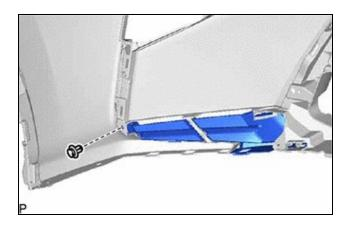
(b) Disengage the claw as shown in the illustration to remove the front bumper arm hole cover LH.
