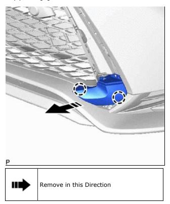
28. REMOVE LOWER RADIATOR GRILLE MOULDING RH (for Mesh Type Radiator Grille)
