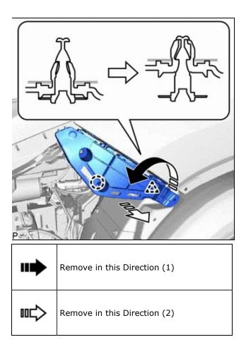
(c) Disengage the claw as shown in the illustration to remove the front bumper side retainer LH.
