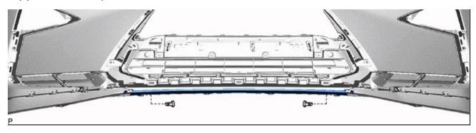
(b) Disengage the 8 claws as shown in the illustration to remove the front bumper guard.
