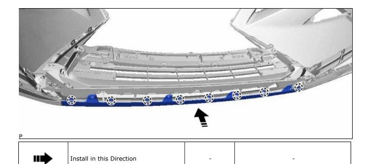
(b) Install the front bumper guard with the 2 clips.
