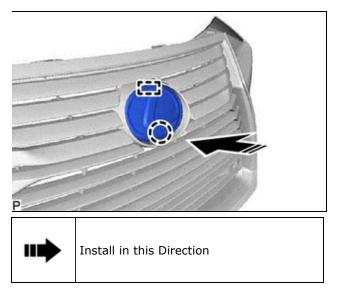
(b) Install the radiator grille (or front panel) emblem with 2 new spring nuts.
