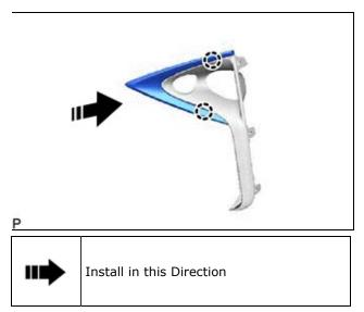
(b) Engage the 5 claws as shown in the illustration to install the fog light cover LH with radiator grille garnish.
