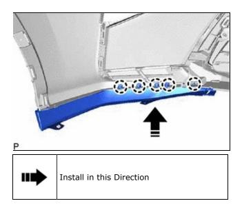
(b) Install the front bumper guard cover LH with the 3 screws.
