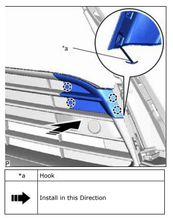
(b) Engage the 4 claws as shown in the illustration to install the front bumper hole cover LH.
