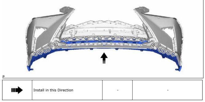
(b) Install the front bumper extension with the 10 screws.
