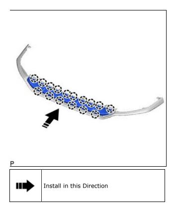
(b) Install the lower radiator grille moulding with the 2 screws.
