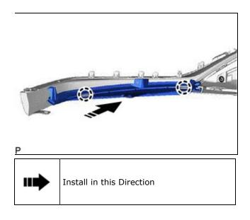
(b) Install the front bumper side support LH with the screw.
