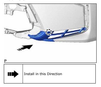
(b) Install the front bumper arm hole cover LH with the clip.
