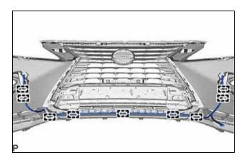
(a) Engage the 9 clamps to install the washer hose.
