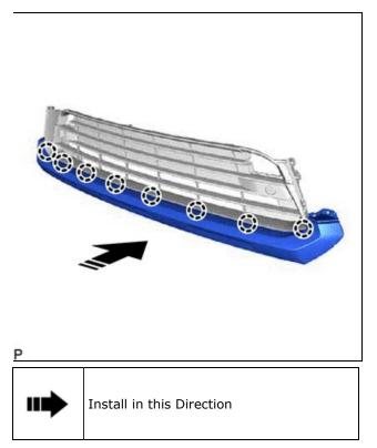
(b) Engage the 5 claws as shown in the illustration to install the lower radiator grille moulding with lower radiator grille.
