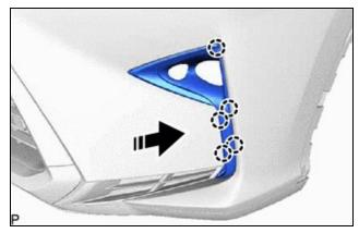
(c) Install the fog light cover LH and radiator grille garnish with the screw.
