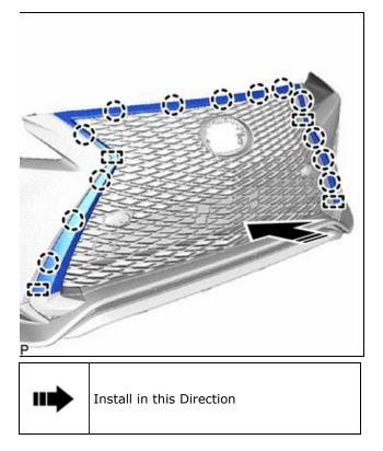
(b) Install the radiator grille moulding with the 6 screws.
