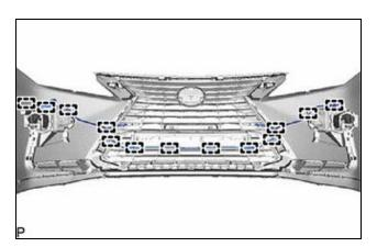
(a) Engage the 13 clamps to install the No. 4 engine room wire.
