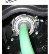
Once the oil stops running out, remove the adapter by twisting it to one side at the hose, then pull it out and set it aside (see illustration).
