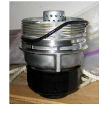
new small "O" ring positioned in groove
