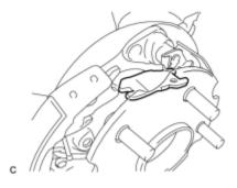
(b) Remove the parking brake shoe strut.
