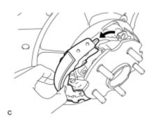
(a) Pull the No. 1 parking brake shoe assembly towards the front of the vehicle by hand as shown in the illustration.
