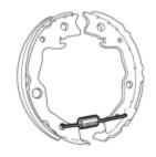
(a) Remove the No. 1 parking brake shoe return tension spring.
