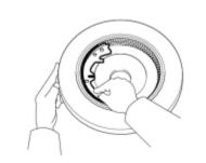
(a) Apply chalk to the inside surface of the disc, then grind down the brake shoe lining to fit the disc.
