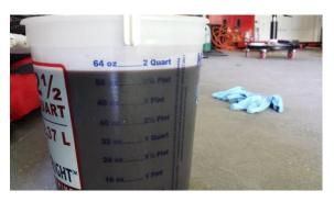
Step 4: Remove the refill plug, replace the aluminum crush washer on the plug. Pump 2 quarts of fresh ATF (ATF-WS) via the refill port. I used my MityVac and poured 6 quarts in the pump reservoir.
