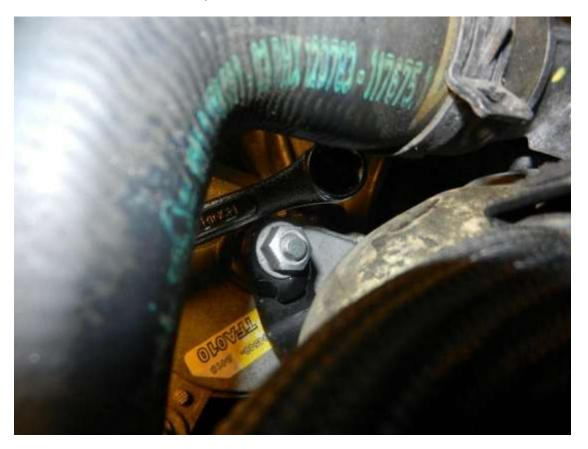
**Step 4:** Get under the car to remove the drain plug, circled red in the picture. Get the pan under it, stick the Allen 5 key on it and unscrew it and let the ATF drain
