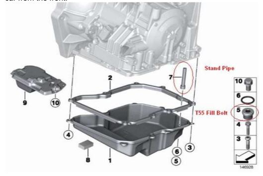
Here is a picture of the drain bolt with the crush washer. After doing the last drain/fill, replace the crush washer for peace of mind and assurance you will not develop an ATF leak. Your dealer should stock it, if not the size in millimeters is 17X12X2.
