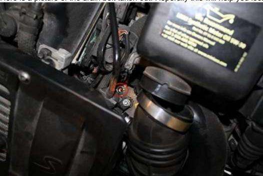
**Step 4:** Get under the car and remove the plastic undertray. You should now be in clear view of the drain plug, circled red in the picture. Get the pan under it, stick the Allen 5 key on it and unscrew it and let the ATF drain
