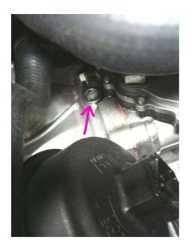
The fill plug with the hex cap and box wrench on top. There is more room on the opposite side from where the wrench is in the photo.
