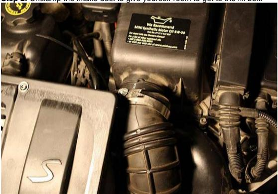
**Step 3:** Put the torx and extensions together and make your way to the fill plug and take it out. A magnet helps a lot holding it from dropping into the engine bay.
