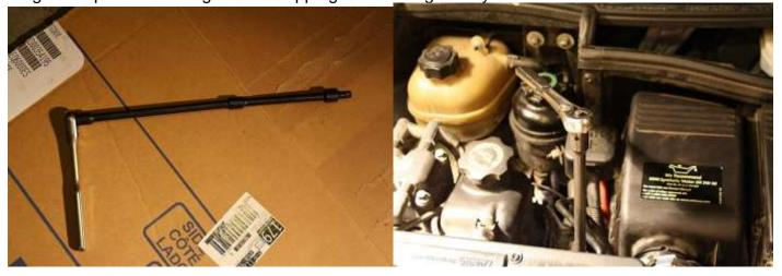
Here is a picture of the drain bolt taken out. Hopefully this will help you locate it in the engine bay
