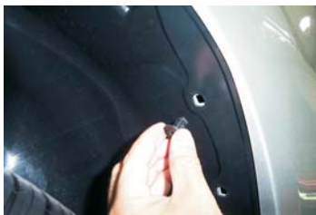
Diagram 3: Remove plastic plugs.
