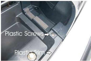
Diagram 1: Remove the Plastic trim.
