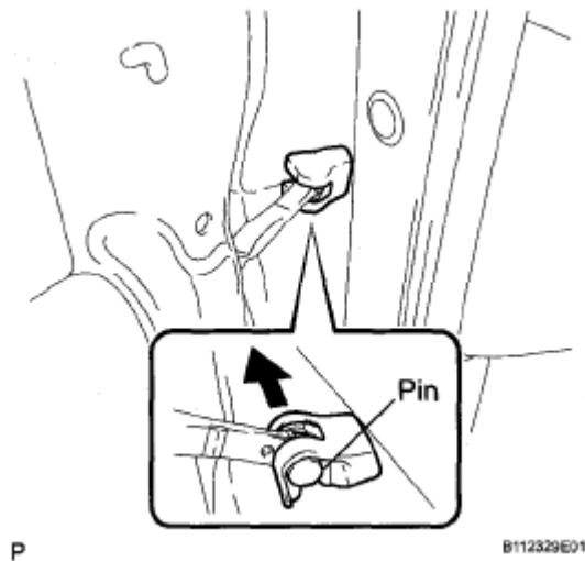
Fig. 120: Identifying Front Door Cover Pin Courtesy of TOYOTA MOTOR SALES, U.S.A., INC.
