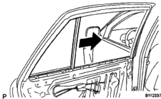
Fig. 144: Removing Rear Door Quarter Window Glass Courtesy of TOYOTA MOTOR SALES, U.S.A., INC.
