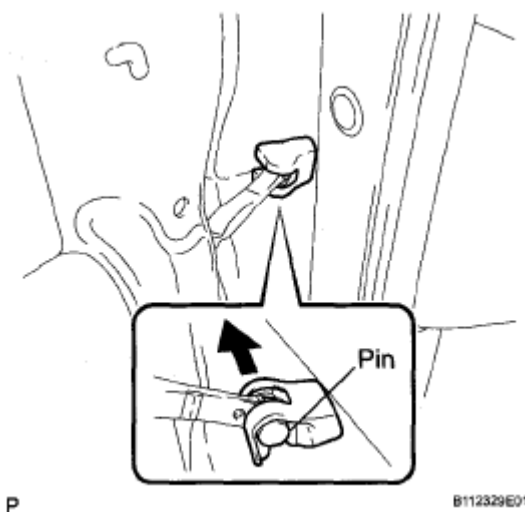
Fig. 156: Identifying Rear Door Cover Pin Courtesy of TOYOTA MOTOR SALES, U.S.A., INC.
