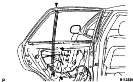
Fig. 143: Identifying Rear Door Window Division Bar Sub-Assembly Bolts And Screw Courtesy of TOYOTA MOTOR SALES, U.S.A., INC.
