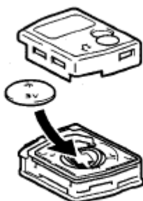
Fig. 75: Installing Transmitter Battery (Lithium Battery) Courtesy of TOYOTA MOTOR SALES, U.S.A., INC.
