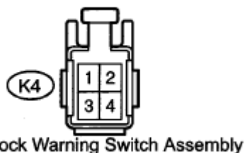
Fig. 72: Identifying K4 Unlock Warning Switch Assembly Connector Terminals Courtesy of TOYOTA MOTOR SALES, U.S.A., INC.
