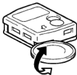
Fig. 74: Prying Transmitter Cover With Coin Courtesy of TOYOTA MOTOR SALES, U.S.A., INC.
