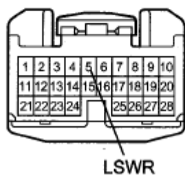
Fig. 25: Identifying Rear Door Lock Assembly & Instrument Panel J/B (Body ECU) Connectors Terminal Courtesy of TOYOTA MOTOR SALES, U.S.A., INC.
