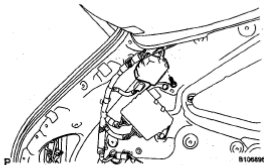
Fig. 94: Identifying Door Control Receiver With Bolt Courtesy of TOYOTA MOTOR SALES, U.S.A., INC.
