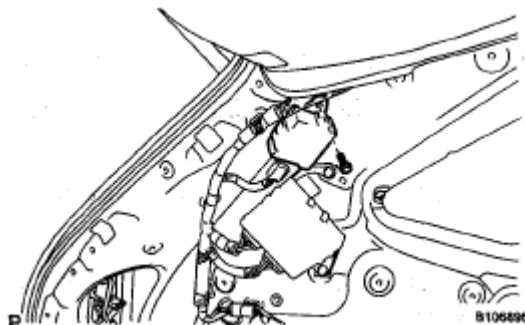
Fig. 93: Identifying Door Control Receiver With Bolt Courtesy of TOYOTA MOTOR SALES, U.S.A., INC.
