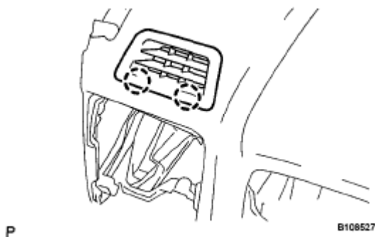
Fig. 32: Identifying Side Defroster No. 1 Nozzle Claws Courtesy of TOYOTA MOTOR SALES, U.S.A., INC.
