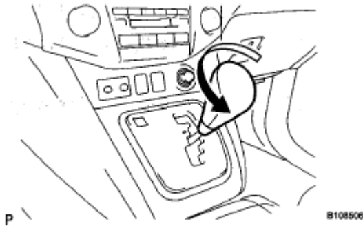
Fig. 10: Identifying Shift Lever Knob Sub-Assembly Courtesy of TOYOTA MOTOR SALES, U.S.A., INC.
