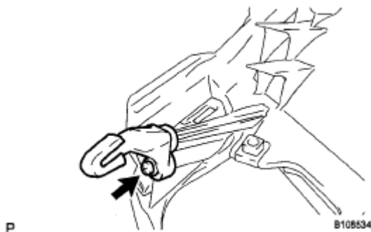
Fig. 47: Identifying Instrument Panel No. 1 Pin Screw Courtesy of TOYOTA MOTOR SALES, U.S.A., INC.
