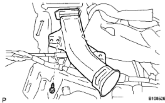
Fig. 43: Identifying Side Defroster No. 1 Nozzle Duct Screw Courtesy of TOYOTA MOTOR SALES, U.S.A., INC.
