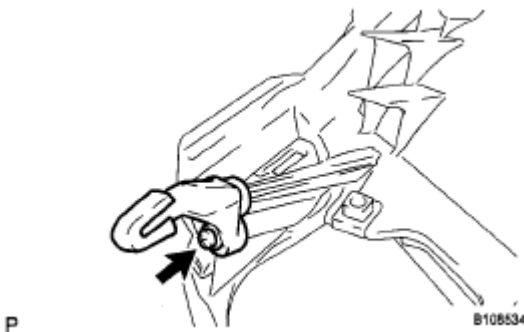
Fig. 27: Identifying Instrument Panel No. 1 Pin Screw Courtesy of TOYOTA MOTOR SALES, U.S.A., INC.
