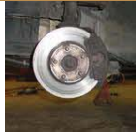
Damaged brake rotor from metal-to-metal contact
