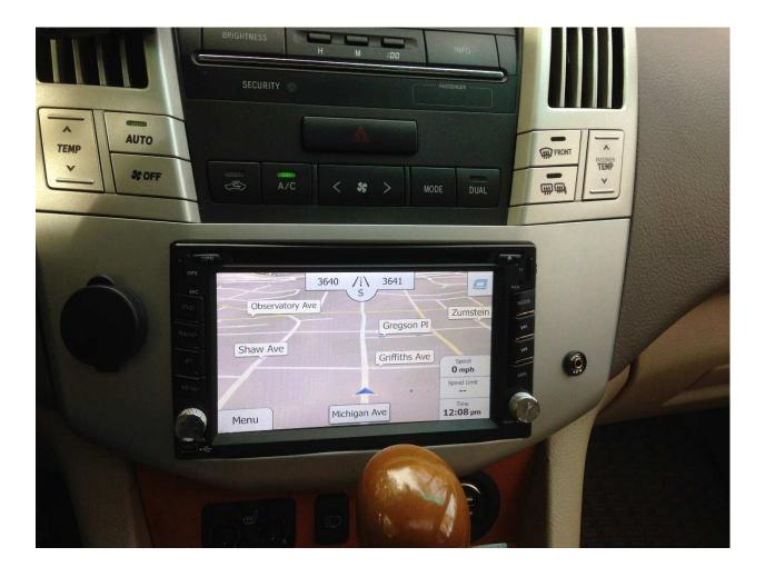
Now that the head unit was mounted and working correctly, I needed to finish the rear camera installation. Recall that I already installed the wireless video receiver when I installed the head unit. Now I needed to mount the camera and install the wireless transmitter to send the video to the head unit when the car is shifted into reverse.
