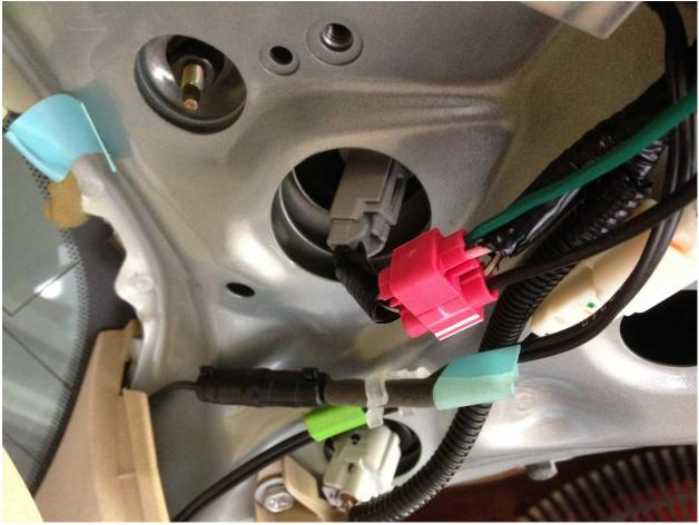
Once the trim was removed, I spliced into the power and ground of the passenger-side reverse light and connected them to the wireless transmitter. The Pink wire is the power (I spliced into it with a Green wire) and the Brown wire is the ground (I spliced into it with a Black wire). The splices are shown in the picture above (red plastic splices).
