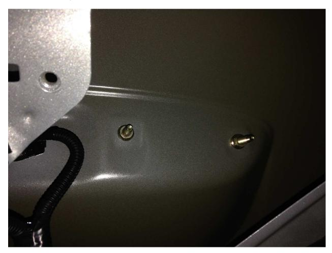
Once the plastic piece is removed, you can see a rubber grommet on the right side of the opening. The camera wire needs to be funneled through it so it can connect to the wireless video transmitter. The grommet already has a cable going through it but there is enough room on the side of the grommet to push the camera wire through. The picture below is looking at the grommet from inside of the car but you will be able to see it from the other side after the plastic piece is removed:
