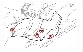
2. Install the No. 1 fuel tank protector with the 4 nuts. Figure 2. Torque: 5.5 N\*m (56 kgf\*cm, 19) in\*lbf)
