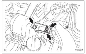
12. Remove the engine moving control rod (dog bone) assembly. Only 3 bolts (28 ft\*lbf) here. Don't make the mistake I did and remove the pivot bolt essentially making this 2 parts instead of 1.
