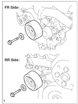
18. Remove the bolt from the tensioner pulley. HINT: This is reverse threaded so loosen it by turning clockwise. I put the engine back down on the mounts for this one and used a flat breaker bar (AutoZone #27115). The manual wants you to remove the whole assembly, but this is impossible
