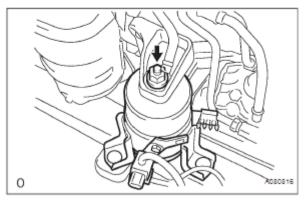
14. Remove the 2 nuts (58 ft.\*lbf) from the RR mounting insulator. This is located back down in the wheel well - back and left of the RH mount.
