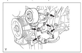
19. With the engine raised again, remove the 4 bolts (15 ft\*lbf) from the water pump pulley. There's special tools for holding the pulley still, but I was able to use leverage from a long (really long) screw driver between the bolts to hold the pulley still. Once they're all cracked loose, back them out by hand. If you left your drive belt on, it should be enough hold without doing anything special. Remove that belt now if you haven't already.
