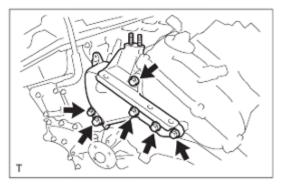
17. Remove the idler pulley bolts (32 ft\*lbf).
