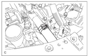
11. Now the fun really starts as we start digging our way towards the water pump. Remove the No. 2 engine mounting stay. There are 2 nuts (17 ft\*lbf) and a bolt (28 ft\*lbf).
