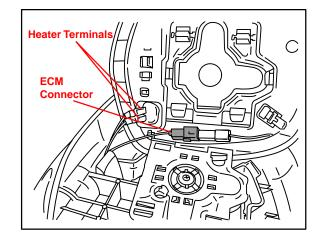
**Repair** 3. Remove the mirror actuator.
