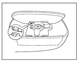
Repair Procedure (Continued) E. Reconnect the mirror holder — Apply pressure to the indicated areas until you hear the holder clips snap into place.
