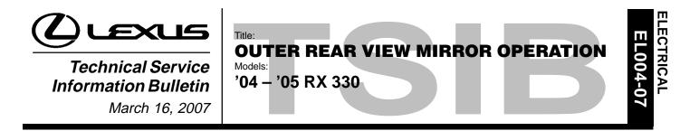
**Introduction** Some 2004 – 2005 model year RX 330 vehicles may exhibit a condition where one or both of the outer rear view mirrors may not operate smoothly from the switch. An updated mirror actuator is available to correct this condition.
