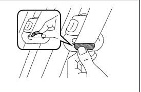
Installation Procedure (Continued) F. By pulling the seat belt up and down several times, as shown in the illustration, securely affix the fluorocarbon resin tape and confirm the smoothness of the belt movement.
