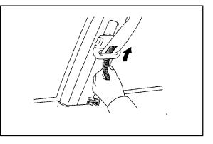
C. Pull both ends of the Velcro tape with your hand and shave off the dirt on the shoulder belt anchor by moving the Velcro tape several times as shown in the illustration.
