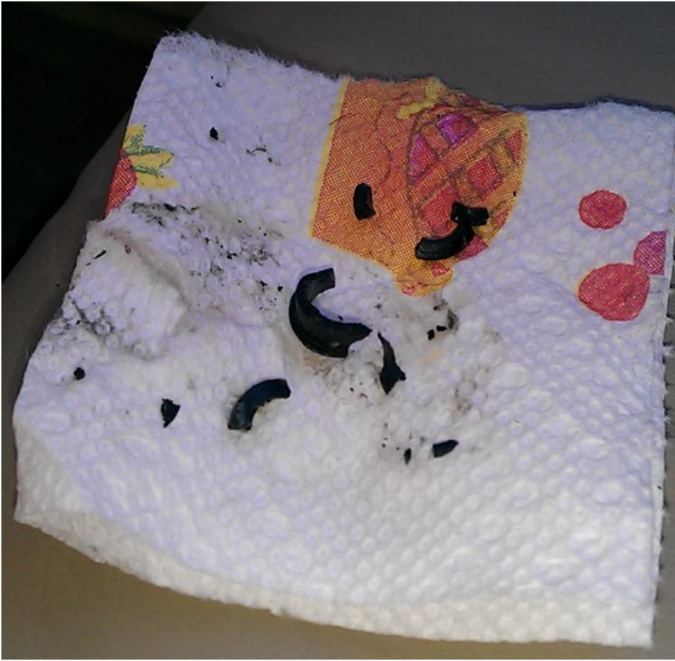
2 - Old shift cable bushing that fell to pieces and left me sitting - IMAG1485
