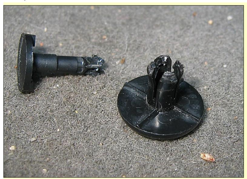
The above photo shows the fastener's two pieces. The fastener base (on the right) locks in when the center piece (left) is inserted and pushed all the way in causing it to spread its 4 sides.
