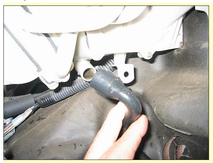
Remove the other end of the tube from the floor hole where the tube exists the floor pan.
