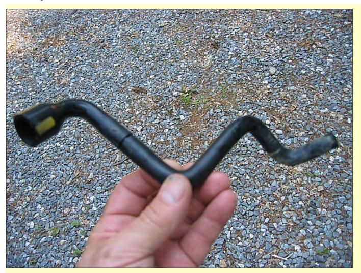
Replace the tube, panel and the fastener holding the panel. The fastener is inserted by first placing the base ring in the hole and then inserting and pressing in the center portion to lock in the fastener.
