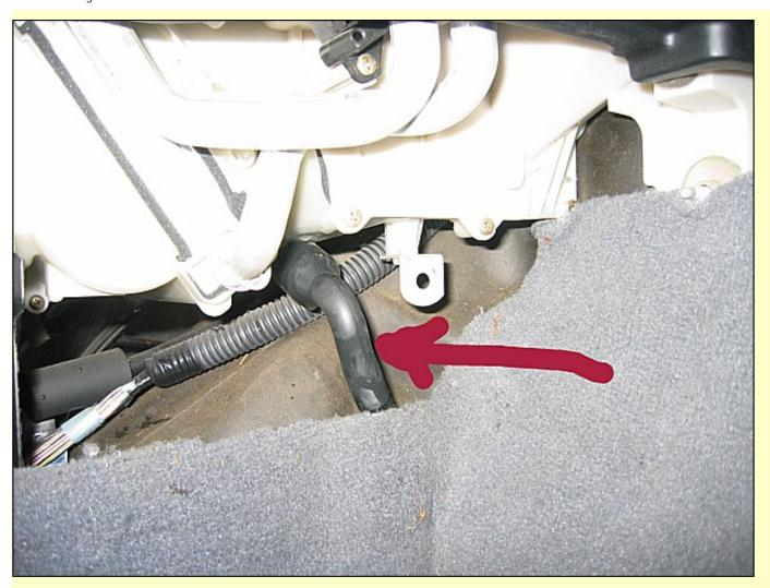
The tube we are looking for is at the bottom of the A/C unit. Pull back the carpet that covers the lower portion of the tube. Disconnect the tube from the A/C unit by pulling it off. Watch - there may be water pouring out of the unit for a second when the tube is removed.
