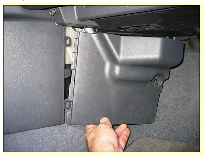
The fastener used in the hole at the right of the panel being removed is a two piece fastener that first requires the center piece to be pried out with a screw driver. Once the center is pried out part way (not necessary to totally remove it from its base), remove the entire fastener from the panel. You may have to apply some elbow grease to pry out the center portion.
