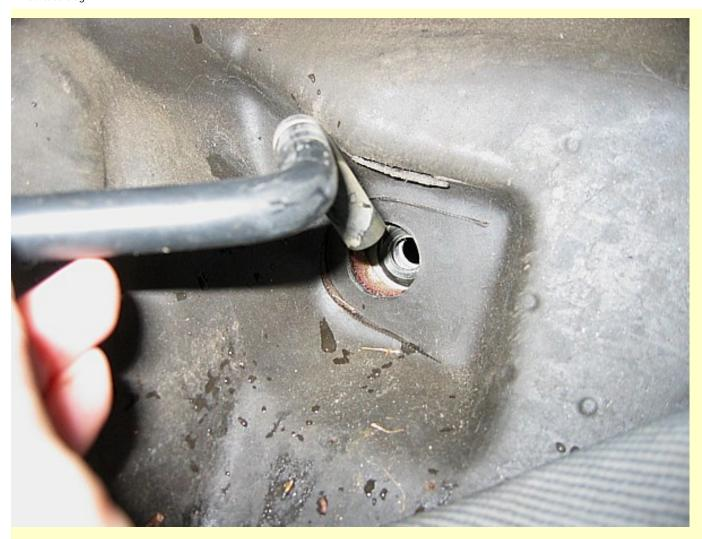
Take the tube out of the vehicle and clean it out. I used a garden hose and put the full force of the water in one end to blow out the blockage. With such sharp bends, no wonder a blockage builds up.
