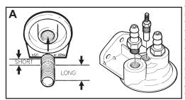
according to the schematic. Install the short end of the threaded nipple into the filter mount and tighten by hand until snug. Wrap a rag around the nipple and tighten with pliers. Squeeze firmly to avoid damage to
