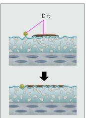
If dirt or foreign matter is allowed to settle and cannot be cleaned off with normal washing, it will be necessary to remove the dirt with the upper layer of the textured finish and then to repaint the entire part.
