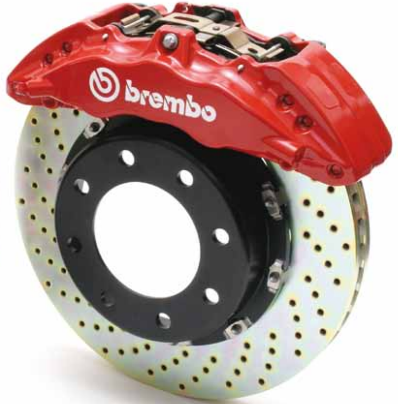
Two-piece "floating" rotor assembly
