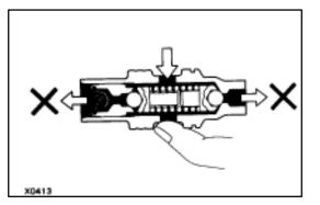
(b) Check the flow control valve for leakage. Close one of the holes and apply compressed air [392-490 kPa (4-5 kgf/cm<sup>2</sup>, 57-71 psi)] into the opposite side, and confirm that air does not come out from the end holes.
