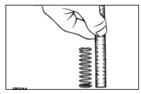
**INSPECT FLOW CONTROL SPRING** 4. Using a scale, measure the free length of the spring. Minimum spring length: 33 mm (1.30 in.) If not within specification, replace the spring.
