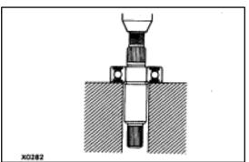
6. IF NECESSARY, REPLACE BEARING(a) Using a press, press out the bearing.
