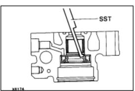
IF NECESSARY, REPLACE OIL SEAL 5. (a) Using SST, tap out the oil seal. SST 09631-10030
