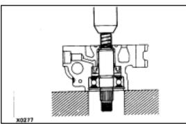
9. REMOVE VANE PUMP SHAFT WITH BEARING(a) Using snap ring pliers, remove the snap ring.
