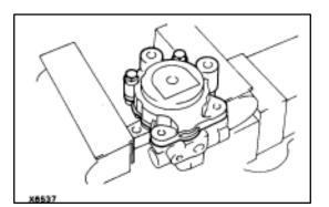
5. REMOVE REAR HOUSING Remove the two bolts and rear housing.
