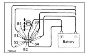
(b) Apply battery voltage to terminal B1 (or B2), and while repeately grounding (\*S4)–(S4 and \*S3)–(S3 and \*S2)–(S2 and \*S1)–(S1 and \*S4) in sequence, check that the valve moves toward the open position.
