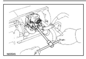
(b) Install the EGR valve with the two nuts. Torque: 18 N·m (185 kgf·cm, 13 ft·lbf)
