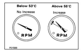
(e) Check whether the engine rpm increases 100–300 rpm under the following conditions.
