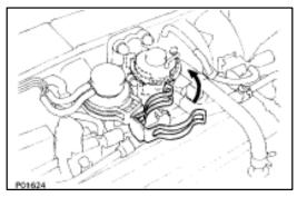
(c) Install the vacuum modulator bracket to the EGR valve.
