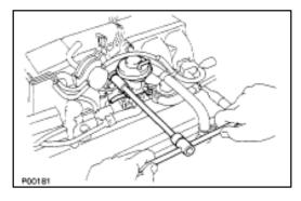
(b) Install the EGR valve with the two nuts.
