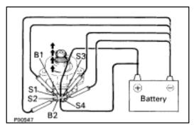
(c) Apply battery voltage to terminal B1 (or B2), and while repeately grounding (\*S1)–(S1 and \*S2)–(S2 and \*S3)–(S3 and \*S4)–(S4 and \*S1) in sequence, check that the valve moves toward the closed position.
