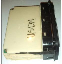
Step 2: Remove the faceplate from your climate controller. There are cable connections between the faceplate onto the controller. One with a large bunch of wires and one with only four wires. The large bunch of wires will stay with the controller and the
