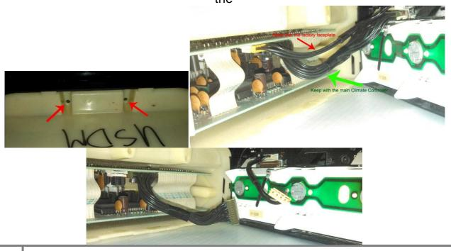
Step 3: Route the OEM cable underneath the main hoop of new Face and plug it into the climate control
