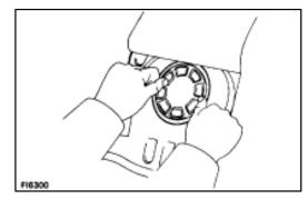
2. **INSTALL PARTITION COVER** Install the partition cover with butyl tape.
