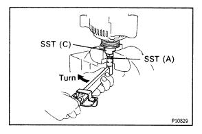
(f) To torque the pulley nut, turn SST (A) in the direction shown in the illustration.
