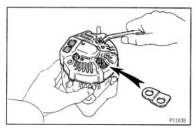
(b) Remove the bolt, 3 nuts, plate terminal and end cover.
