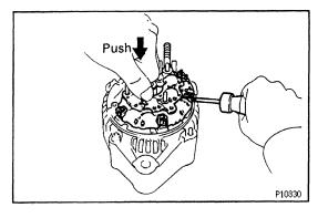
(b) Install the rectifier holder while pushing it with the 4 screws.
