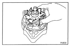
2. INSTALL ROTOR TO RECTIFIER END FRAME
