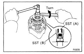
(g) Turn SST (B), and remove SST (A and B).
