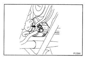
(e) Remove the bolt, nut, pipe bracket and generator.
