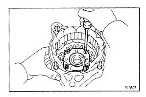
(d) Install the bearing retainer with the 4 screws.
