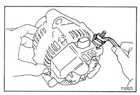
(b) Install the terminal insulator with the nut. Torque: 6.5 N-m (66 kgf-cm, 58 in.-lbf)
