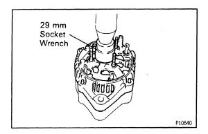
(b) Using a 29 mm socket wrench and press, slowly press in the rectifier end frame.
