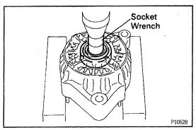
(b) Using a socket wrench and press, press out the bearing.
