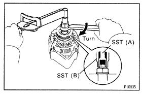
(b) Hold SST (A) with a torque wrench, and tighten SST(B) clockwise to the specified torque.SST 09820-63010
