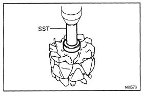
(b) Using SST and a press, press in a new bearing. SST 09820-00030
