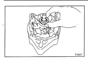
(c) Remove the generator washer.
