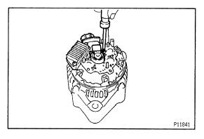
(b) Remove the 5 screws, brush holder and voltage regulator.
