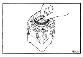
(h) Remove the pulley nut and pulley.
