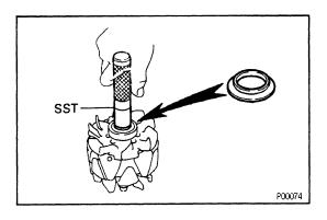
(c) Using SST, push in the bearing cover. SST 09285-76010
