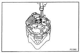
(b) Place the voltage regulator and brush holder on the rectifier end frame.
