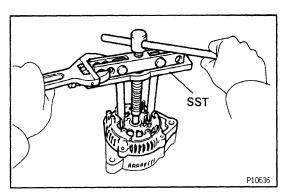
(b) Using SST, remove the rectifier end frame. SST 09950-20017
