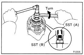
(h) Turn SST (B), and remove SST (A and B).
