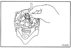
(c) Remove the seal plate from the rectifier end frame.
