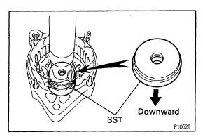
(c) Using SST and a press, press in a new bearing. SST 09608-20012 (09608-00030)
