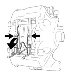
(b) Push the pin hold clip toward the brake rotor to disengage it from the brake pad, and then remove it from the 2 pad guide pins.
