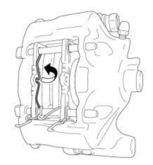
(c) Holding the anti-squeal spring, remove the 2 pad guide pins from the rear disc brake cylinder assembly.
