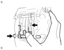
(d) Holding the anti-squeal spring, install the pad guide pin (lower) to the rear cylinder assembly.
