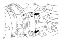
(b) Install the cylinder assembly rear together with the caliper support bracket with the 2 bolts.
