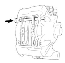
(c) Insert the end of the anti-squeal spring to the brake pad (inner).
