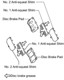
(a) Apply disc brake grease to both sides of the 2 No. 1 anti-squeal shim.
