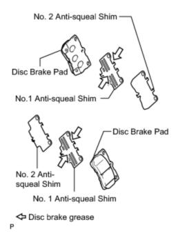
(a) Apply disc brake grease to both sides of the 2 anti-squeal shims.
